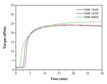
**Figure 1.** Isothermal vulcanization curves of the rubber mixtures.
