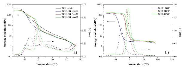
Figure 4. Thermomechanical curves of a) the TPU matrix and the TDVs, and b) the rubbers.
